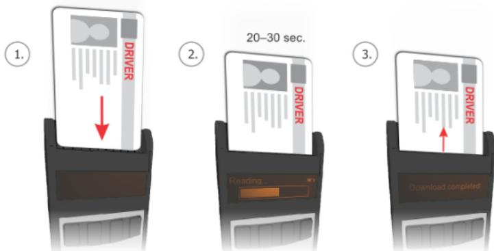
In order to make a driver card download with the device you have to insert the driver card into the card slot of the device in the way shown in picture.
