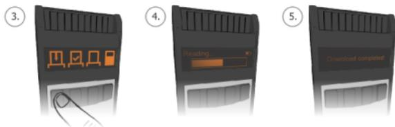
By pressing **F2** you can choose which records to download. Function buttons can have different functions in sub menus, their functions are shown in lower part of display.
