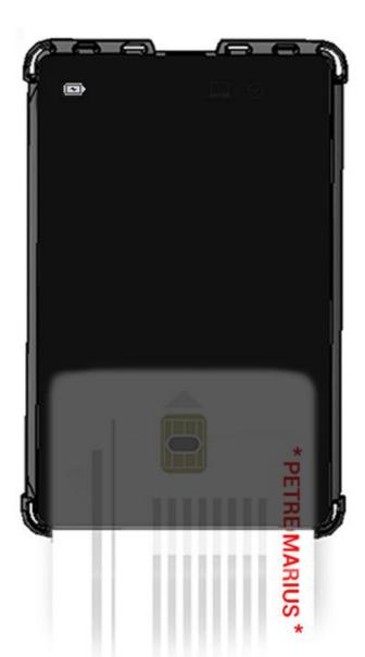
Note: if the **battery level indicator blinks**, you'll be able **to download a few files only**, as you **need to charge** the device soon.
