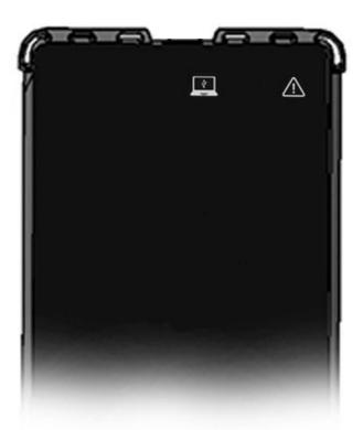
Note: if the **PC** and **warning indicators are blinking inter- mittently**, the **device is low on storage space**.
