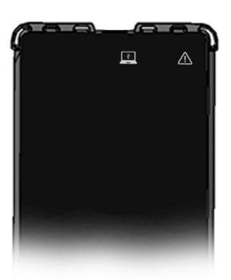
Note: if the **PC** and warning indicators are blinking simultaneously, the device's storage is full. You will need to delete some files.
