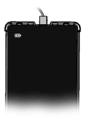
Note: if the **battery level indicator is blinking** your device **is in charging mode**.
